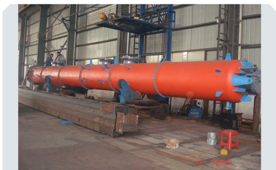
脱硫塔/Desulfurization Tower 规格/Specification: OD1200mm X 12mm X 16800mm
