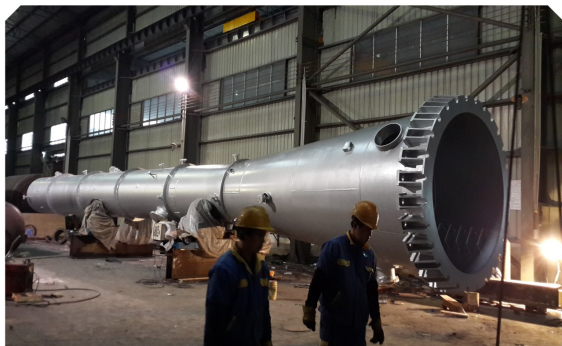
T-702抽提蒸馏塔下段 T-702 Extractive Distillation Column (塔体共分三段 总长54.428米) / The body of the column is divided into three parts, and the above image shows the bottom part. (Total length of the column: 54.428m)
