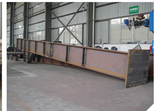
图为厂房钢结构的一部分: 金字梁 (左) 和立柱 (右) These two pictures are constituent parts of the steel structure factory building:crossbeam(left)and pillar(right).
