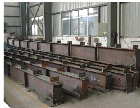
图为厂房钢结构的一部分: 金字梁 (左) 和立柱 (右) These two pictures are constituent parts of the steel structure factory building:crossbeam(left)and pillar(right).
