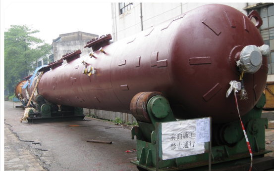
溶剂回收塔/Solvent-recovery Column 规格/Specification: OD1600mm X 16mm X 20000mm
