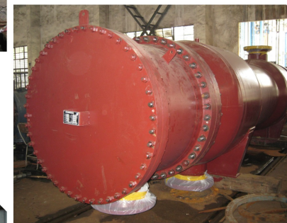
冷凝器/Condenser 规格/Specification: OD3800mm X 20mm X 12000mm
