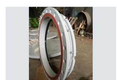
不锈钢双法兰同心锥管/ Stainless Steel Concentric Reducer 规格/Specification:OD405mmX400mm(高/H)
