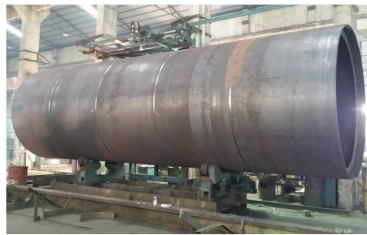
大桩管/ Large pipe pile bottom through 型号: OD3200mmX25mm厚(thk)X10000mm
