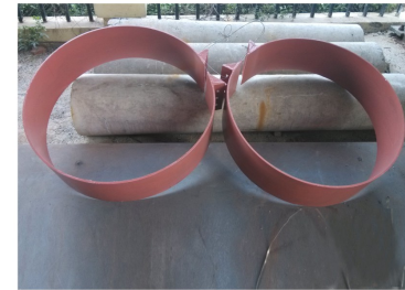
DN800管环/Mild Steel Split Collar 规格/Specification: OD833mmX8mm(厚/Thk)X250mm(高/H)
