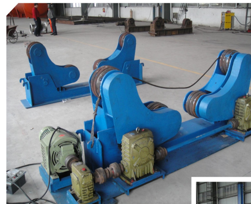
滚轮架/Roller carrier 型号: ZN-20t
