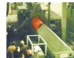
Centrifugal casting Machine (for DN700-DN1200 mm pipe)
