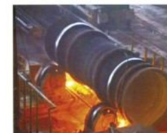
Centrifugal casting Machine (for DN700-DN1200 mm pipe)
