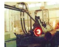
Centrifugal casting Machine (for DN100-350 mm pipe)
